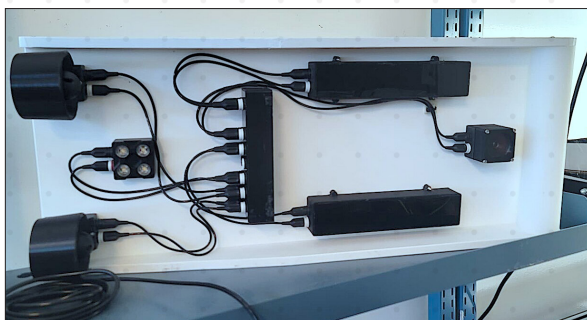
Underbelly showing the modular components in place using Bristlemouth connectors
